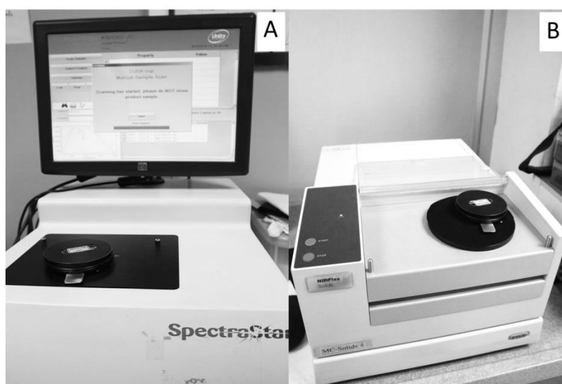
Figure 1. The same anti-acne gel sample was carried on to collect the NIR spectra using a grating NIR spectrophotometer model SpectraStar™ 2500 (A) and a FT-NIR spectrophotometer model NIRFlex N-500 (B).
